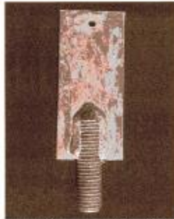
PSA Strap Anchor J-Type Finish after 360 hrs.
