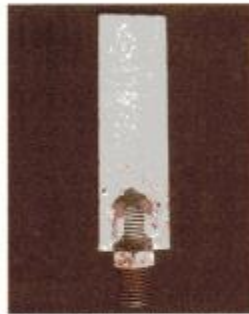
PSA Strap Anchor Hot Dip Galv. Finish after 360 hrs.
