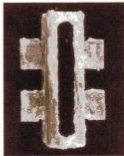
PSA Insert (Top) Hot Dip Galv. Finish after 648 hrs.
