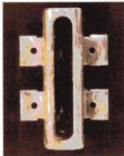
PSA Insert (Top) J-Type Finish after 648 hrs.
